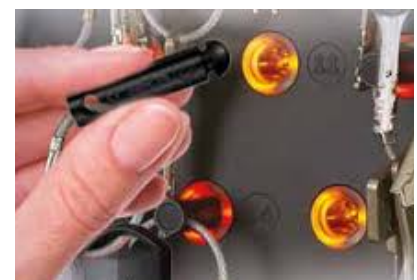
Amber light indicates correct return key position for easy returning of keys back
